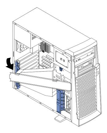
Complete the following steps to remove the support bracket assembly:
